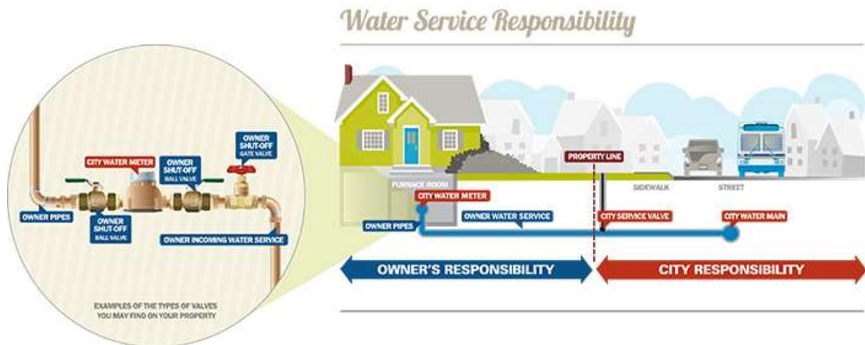
Homeowners are responsible for water lines from the curb stop (city service valve) to the house. The Village is responsible for water lines from the curb stop (city service valve) to the main water system.
