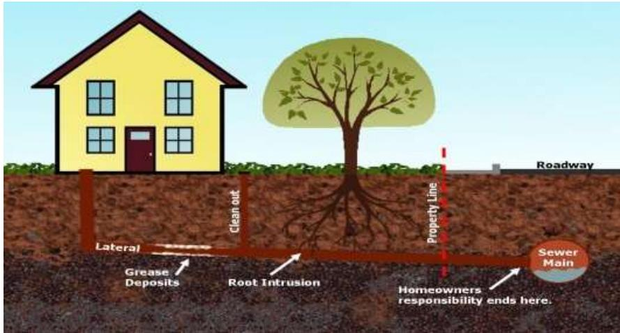
Homeowners are required to maintain the lateral from their home, to the main sewer line, typically located in the street or nearby easement. Maintaining the lateral includes keeping the lateral line flowing and free of debris such as roots, or grease.
